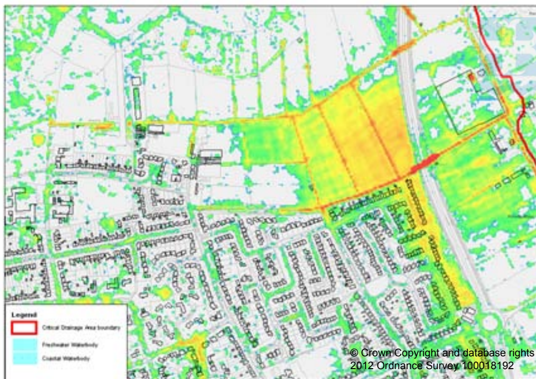
Figure E-4: Flooding in Hawksworth Drive area from Wham Dyke, Acre Lane Brook and Eight Acre Lane
