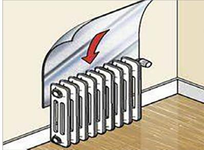
*Cutting the foil to size will mean it is not visible in the room*
