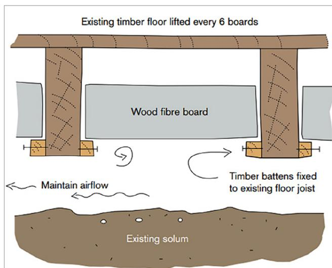
*Air flow should be maintained to prevent moisture build up and rotting*
