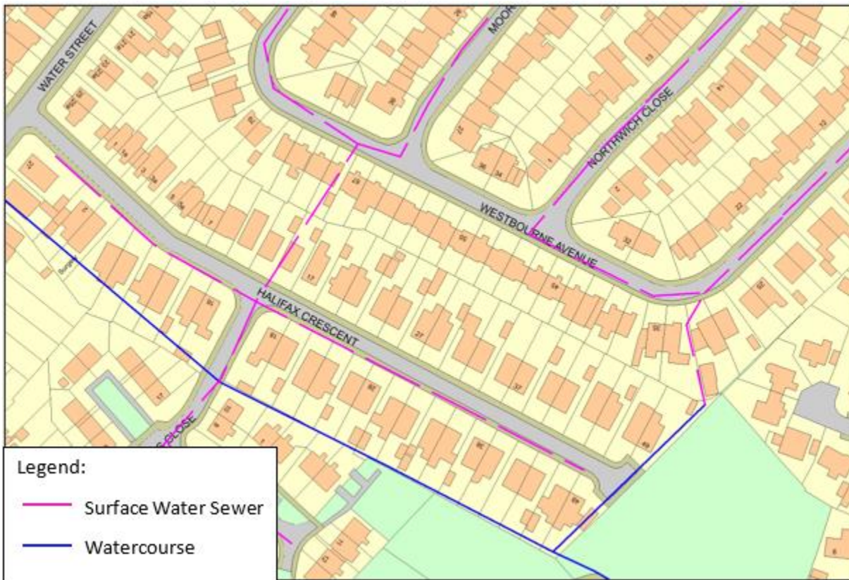
Figure 2 Surface water drainage network
