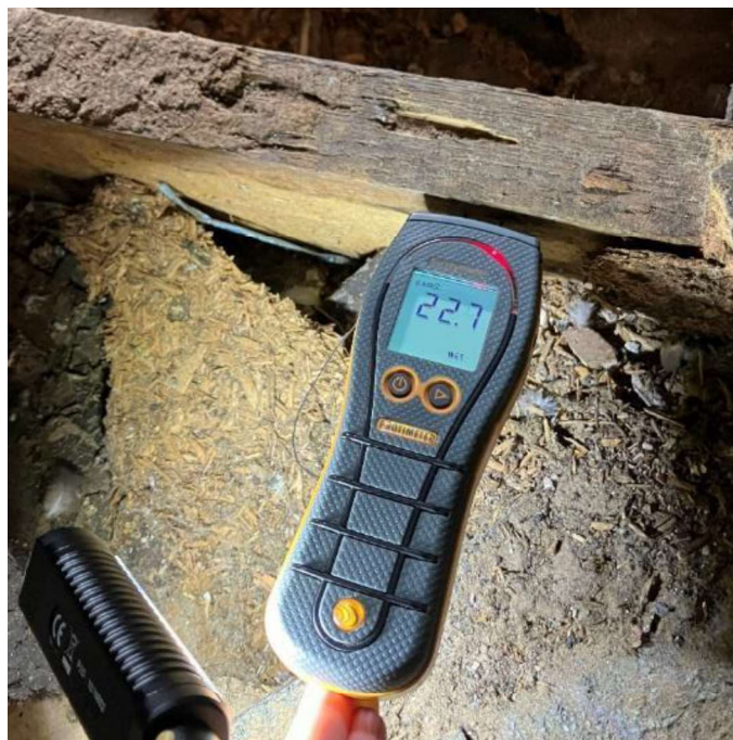
Figure 58: Moisture metre reading of timber floor joists.
