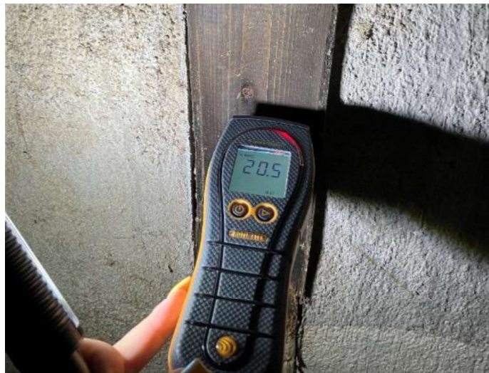
Figure 54: Moisture reading of exposed timbers to internal walls.
