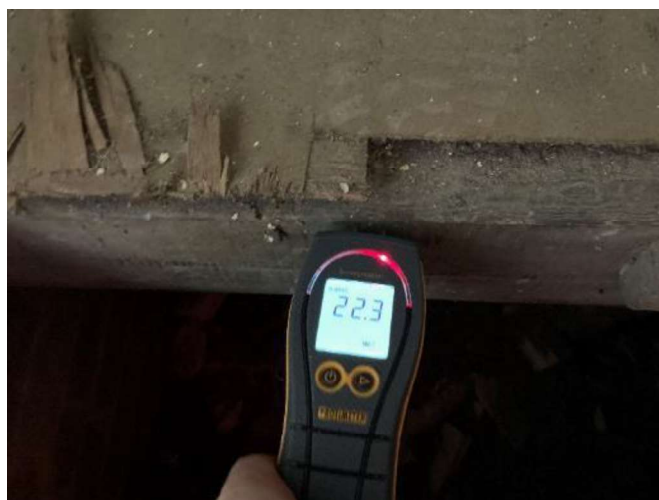
Figure 38: Moisture reading of ground floor timber floor joists.
